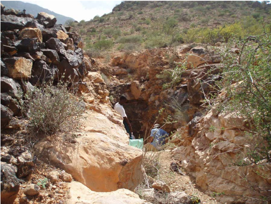
Figure 2: Old Exploration Adit at Qandala. Note the massive iron rich gossan on the mullock dump. A literature study suggests that there are many geological similarities between the style of mineralisation at Jabali and that seen at Qandala.
